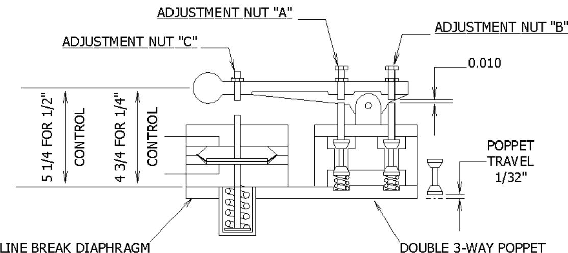
When replacing poppets, it is essential that poppet travel be  $1/32$  inch. Less than this will cause leakage of power gas to the exhaust. More than this amount will cause the poppets to be crushed and will eventually cause leakage. Poppet pins may have to be lengthened or shortened to insure this  $1/32$  inch travel. Poppet pins may be made from  $1/4$  inch stainless steel round bar.
