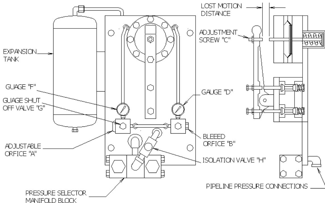
5. To determine the adjustable orifice setting, subtract the final pressure reading from the initial pressure reading and divide by five. Example:
