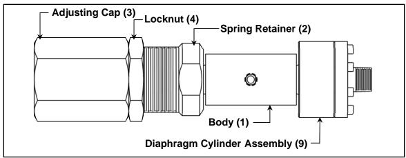
Figure 1: Air Relay Valve with 1-1/4 Diaphragm
