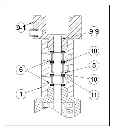
Figure 7: Installing Cylinder
