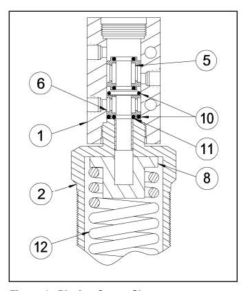
Figure 4: Placing Center Sleeve
