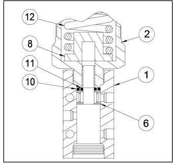
Figure 3: Installing Spring Retainer
