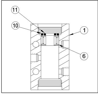
Figure 2: Placing End Sleeve Seals
