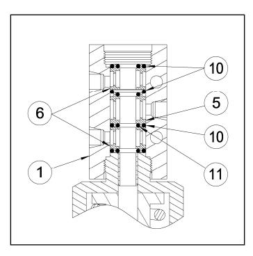
Figure 6: Placing Last End Sleeve
