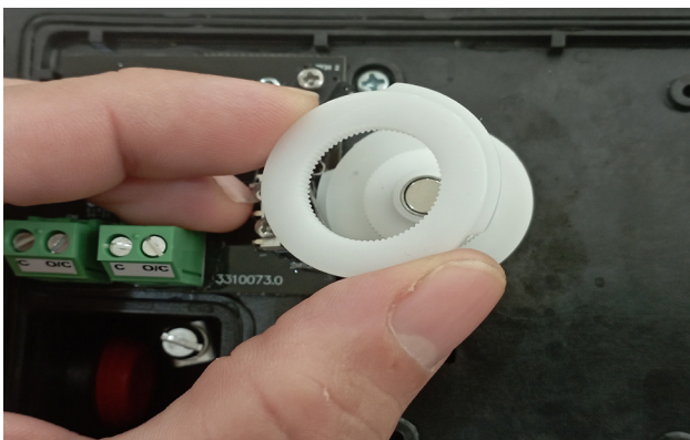
Figure 7-17 Removing the Top CAM
