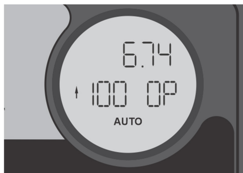
Figure 8-39 Closing Time Stored in Calibration
