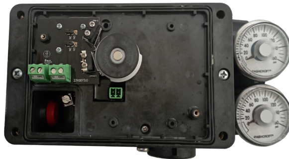
Figure 7-11 View of Jumpers and Cams
