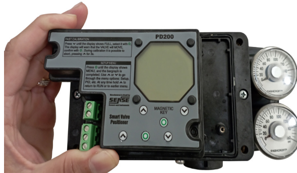
Figure 7-10 Pulling off the Internal Cover
