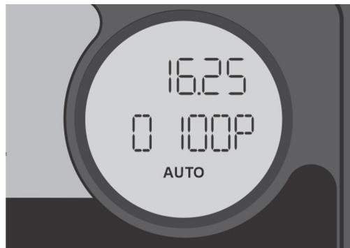
Figure 8-38 Opening Time Stored in Calibration
