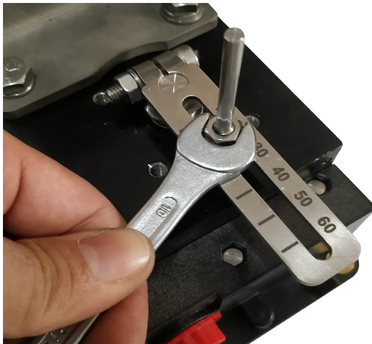
Figure 5-20 Installing the Dowel Pin
