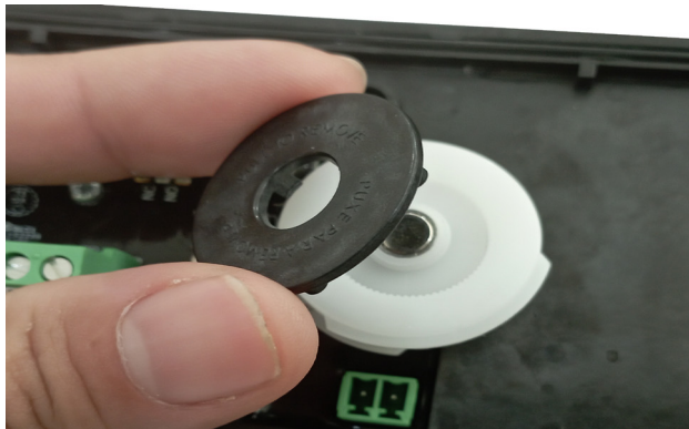
Figure 7-16 Removing the Lock
