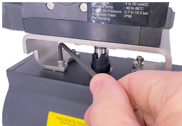
Figure 5-8 Tightening the Bracket Bolts
