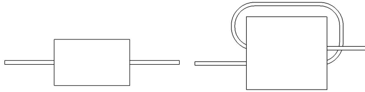
Figure 2-9: Small ferrite beads in I/O wiring
