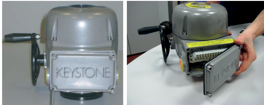
Figure 3 Removing terminal board enclosure cover
