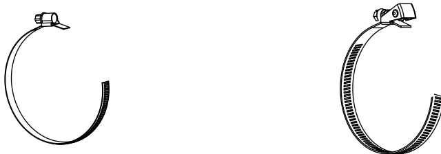
Fig. 6.38: Band clamp clasp with tension strap Fig. 6.39: Quick release clasp with tension strap
