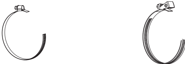
Fig. 6.36: Band clamp clasp with tension strap Fig. 6.37: Quick release clasp with tension strap
