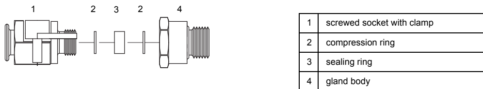
Fig. 8.7: Cable gland for mines M25
