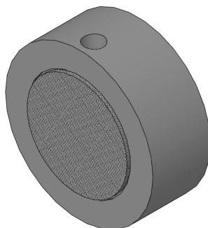
Figure 1-4: Snubber Diffusion Assembly
