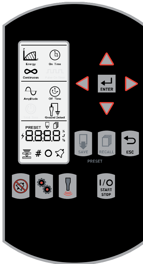
Figure 6.1 LPX Power Supply User Interface
