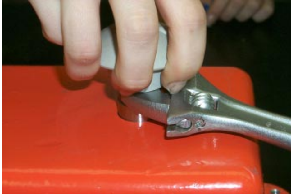
Manual Declutch On 300 and 500 Series
