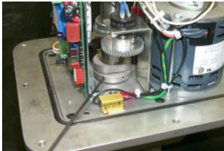
Cam Setting For All Actuators
