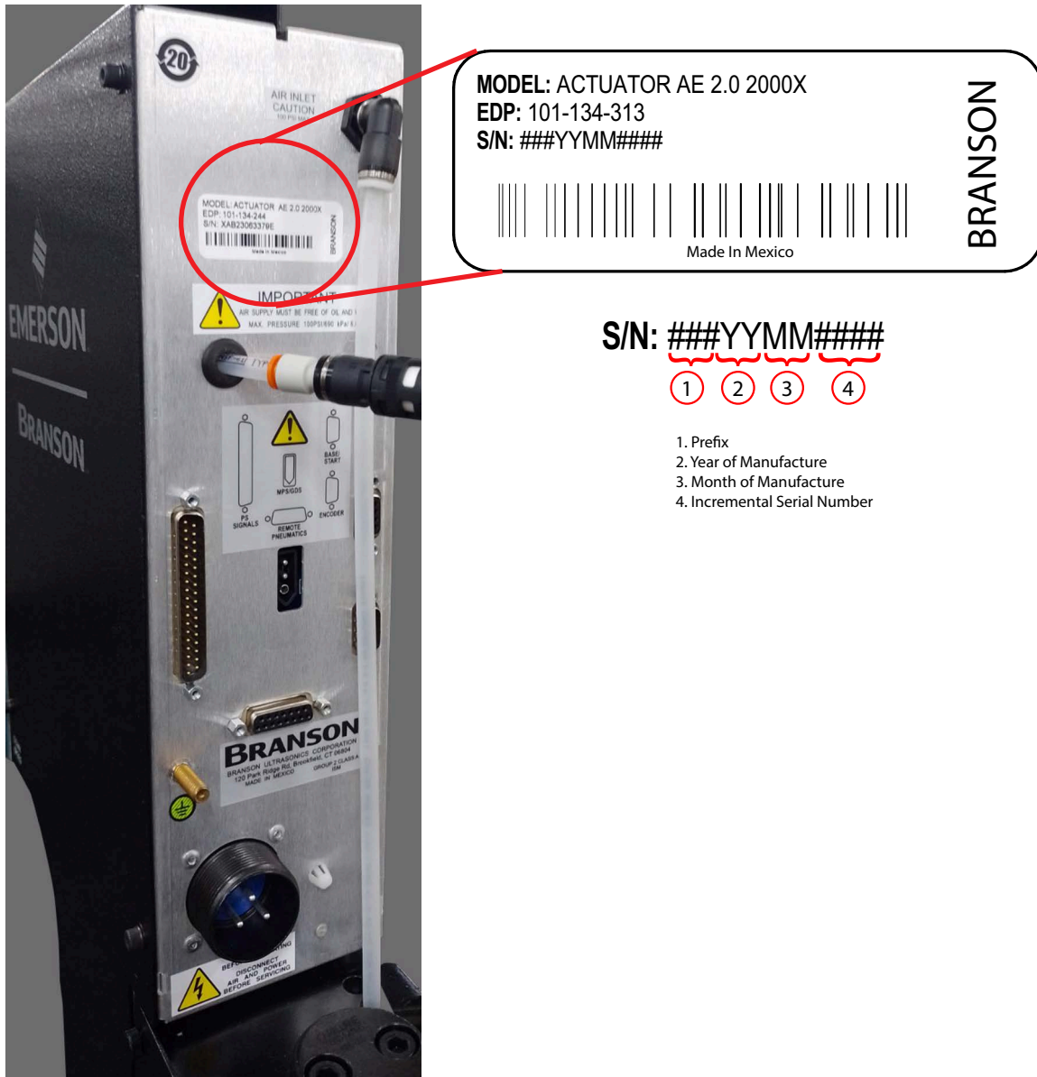
Figure A.1 Location of the information Label in the 2000X Power Supply
