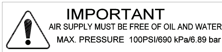
Figure 1.3 Caution label on the 2000X aed Actuator for the factory air supply
