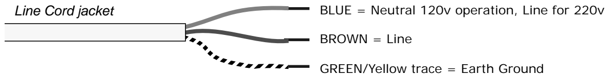
Figure 4.13 International Harmonized Line Cord Color Code
