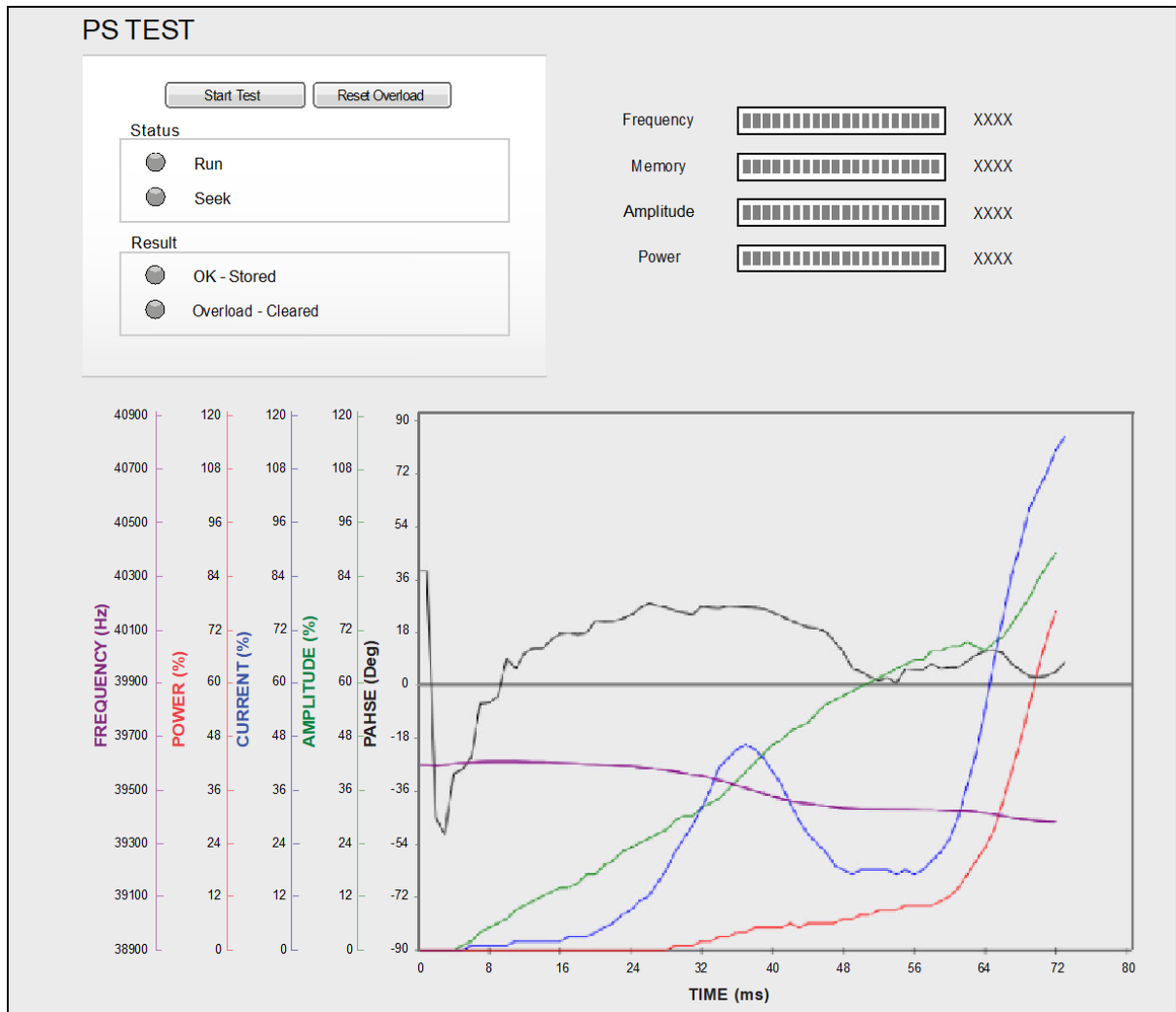
Figure A.10 Weld Graph, Defective Horn
