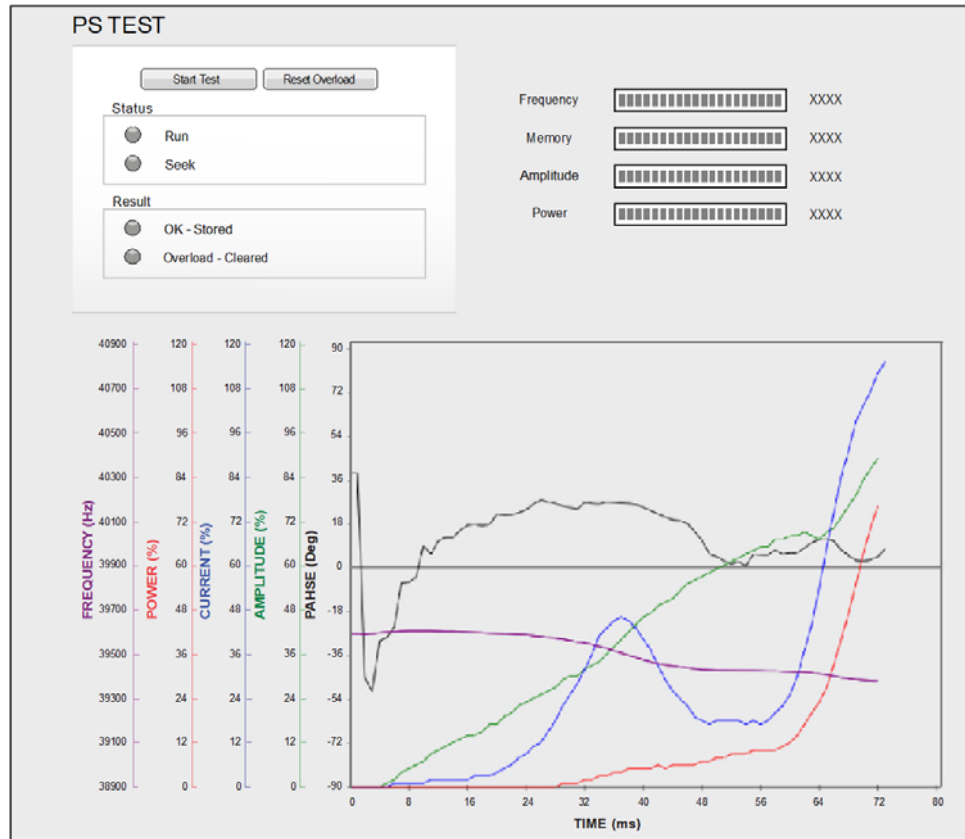
Figure A.11 Weld Graph, Defective Converter
