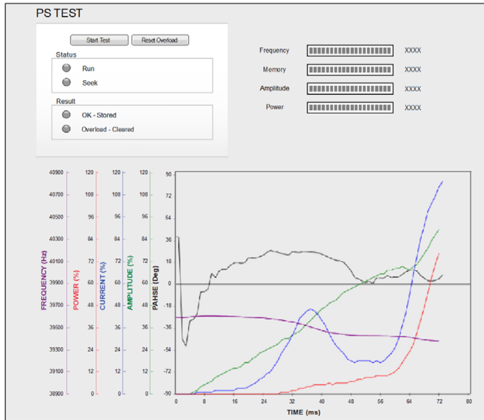
Figure A.10 Weld Graph, Defective Horn
