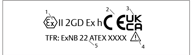
Fig. 3: Name plate for mechanical explosion protection
