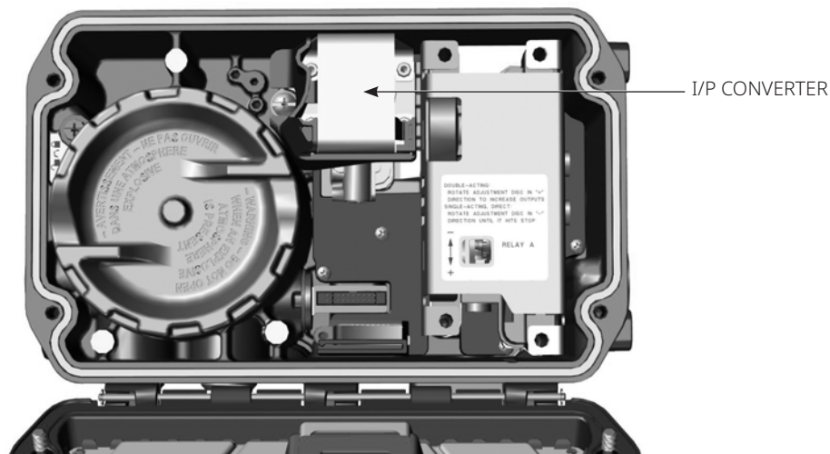
Figure 12. I/P Converter Location
