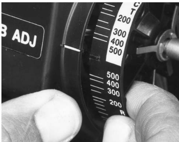
Figure 3-2. Changing Controller Action (Fisher 4194A Controllers)
