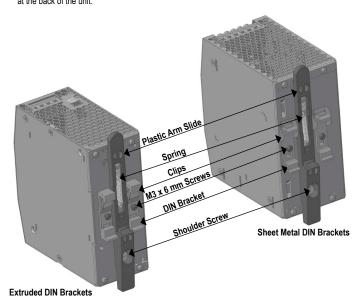
Retain / Slide the two DIN brackets back of the unit. Place the Panel Mount Bracket on top of the DIN Brackets. Use the DIN Bracket to align the Panel Mount Bracket in the mounting hole. Affix the Panel Mount Bracket using the included M3 x 8mm Phillip screw. Recommended torque is 6lbf-in (7kgf-cm).
