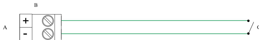
Figure 4-25: Discrete input wiring (internally powered)
