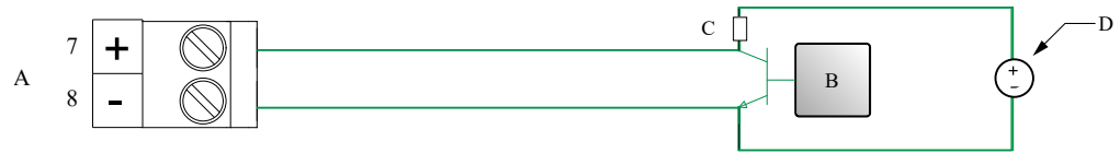
Figure 4-28: Frequency input wiring (externally powered)
