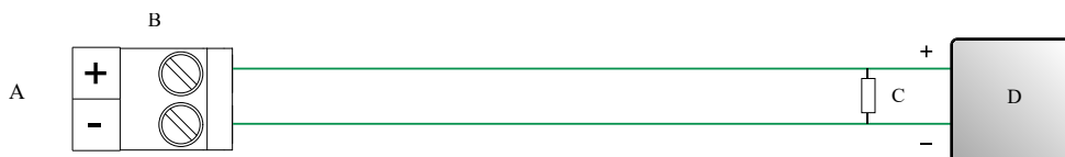
Figure 4-3: mA output wiring (internally powered)
