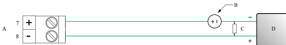
Figure 4-15: Frequency output wiring (externally powered)
