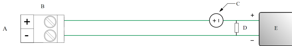
Figure 4-12: Frequency output wiring (externally powered)
