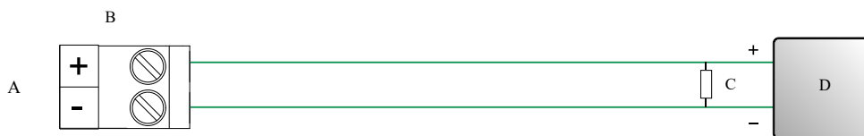
Figure 4-10: Frequency output wiring (internally powered)
