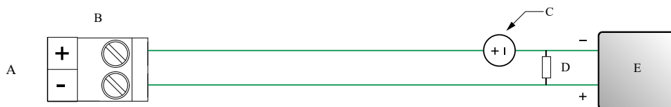
Figure 4-18: Discrete output wiring (externally powered)
