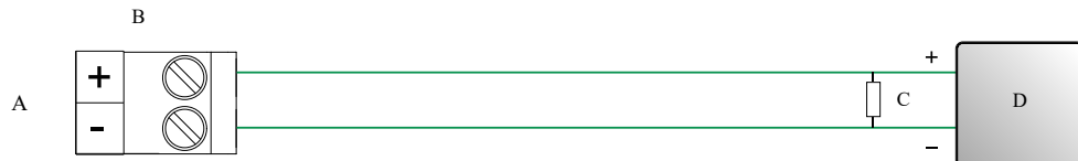
Figure 4-16: Discrete output wiring (internally powered)
