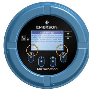
Figure 9-3: Example 2: Active arrow indicators on the transmitter display
