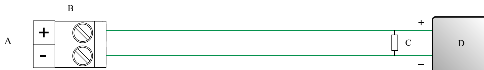
Figure 4-1: Internally-powered mA Output wiring
