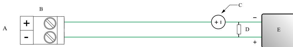
Figure 4-2: Externally-powered mA Output wiring
