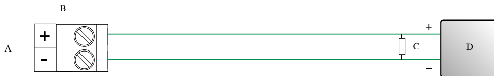
Figure 4-7: Internally-powered DO wiring
