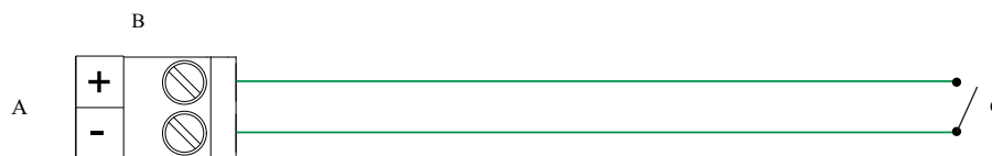
Figure 3-20: Discrete input wiring (internally powered)
