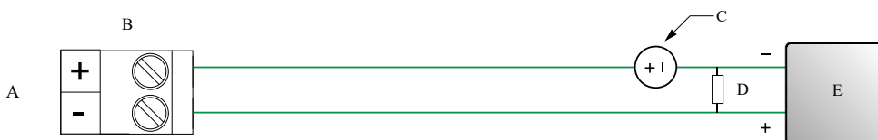
Figure 4-4: Externally-powered DO wiring
