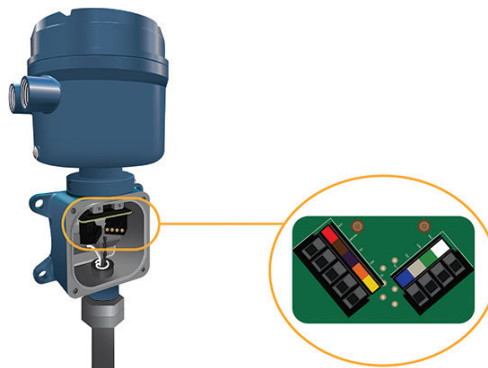
Figure 3-4: 9-wire transmitter-to-sensor wiring connections
