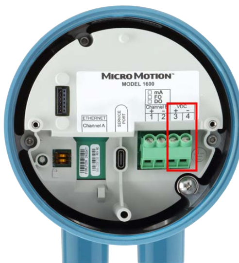
Figure 5-1: Location of power supply wiring terminals and equipment ground
