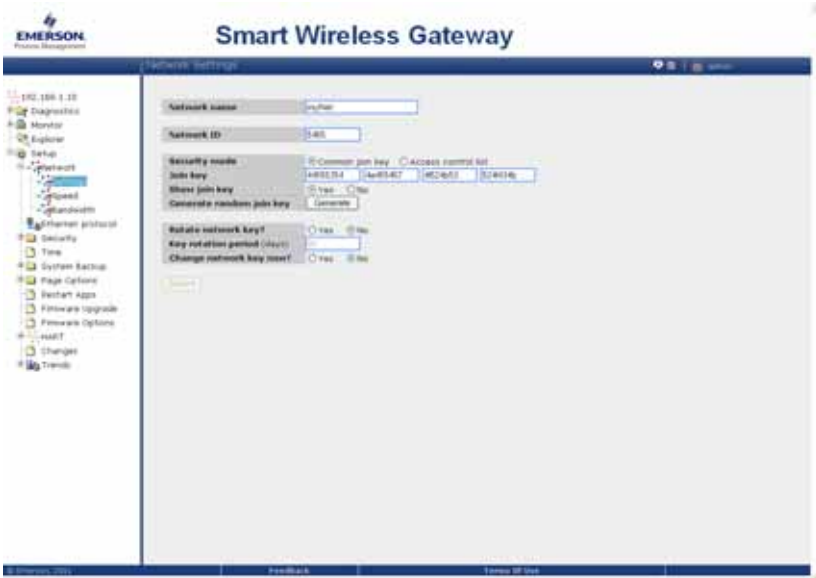
Figur 13. Nettverksinnstillinger for Smart Wireless Gateway
