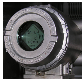
Figure 1-8: Optional local display and glass endcap
