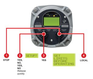
Place the selector knob in the **STOP** position. Then toggle the control knob in rapid succession to **YES**, then **NO**, then **YES**, then **NO** and release. The Setup icon will be displayed on the display module and "SETUP?" will be displayed on the message center. Rotate the control knob to "YES." The message center will display "SET LIMITS BEFORE OPERATING." Set position limits as described on the next pages.
