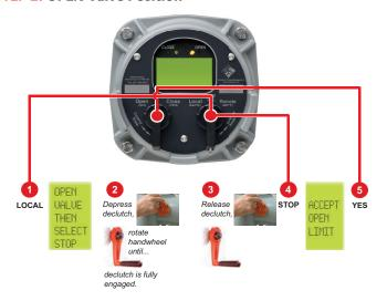
Turn the selector knob to the LOCAL position. At the "OPEN VALVE THEN SELECT STOP" prompt, depress the declutch lever while rotating the handwheel until the clutch is fully engaged. Release the lever. When the valve is fully opened. Return the selector knob to the STOP position. At the "SAVE LIMITS" prompt, select "YES." Advance to the "SAVE CHANGES?" prompt and answer YES to save the changes.
