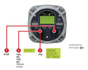
Turn the selector knob to the **STOP** position then toggle the control knob in rapid succession to **YES**, then **NO**, then **YES**, then **NO** and release. The setup icon will be displayed on the display module and "SETUP?" will be displayed on the message center. Rotate the control knob to **YES**. The message center will display "CHANGE DISPLAY SETTINGS"
