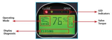
Once you follow the simple steps outlined in this guide, the actuator will be ready for normal operation. The bar graph, position digits, icons, and LEDs will indicate the valve status.
