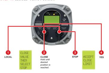
Turn the selector knob to the "LOCAL" position. Hold the control knob in the "CLOSE" position until desired position is reached. Dis-engage motor drive by setting the declutch lever in "HAND" mode. Using handwheel, move the valve in the open direction for one handwheel turn to allow for motor coasting. Re-engage motor drive by setting the declutch lever out of "HAND" mode. Return the selector knob to the "STOP" position. Select "YES" to set new close limit.
