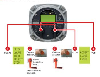
Turn the selector knob to the **LOCAL** position. At the **"CLOSE VALVE THEN SELECT STOP"** prompt, depress the **declutch lever** while rotating the **handwheel** until the clutch is fully engaged. Release the lever. When the valve is fully closed. Return the selector knob to the **STOP** position. At the **"ACCEPT CLOSE LIMIT"** prompt, select **"YES."** Advance to the **"SAVE CHANGES?"** prompt and answer **YES** to save the changes.
