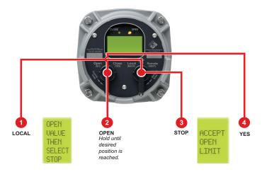
Turn the selector knob to the "LOCAL" position. Hold the control knob in the "OPEN" position until desired position is reached. Dis-engage motor drive by setting the declutch lever in "HAND" mode. Using handwheel, move the valve in the close direction for one handwheel turn to allow for motor coasting. Re-engage motor drive by setting the declutch lever out of "HAND" mode. Return the selector knob to the "STOP" position. Select "YES" to set new open limit.
