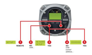
In the "SETUP" mode advance to "NETWORK SETUP?" using the selector knob in the REMOTE position. Answer YES. Hold the control knob in the NO position until the correct address appears. Answer YES. Unit is now network controlled. If other configuration changes are needed, please see the TEC2 Installation & Operation Manual (EZK-420-0117), which can be found at www.emerson.com/eim.
