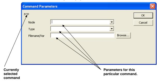
Figure 2-11. Command Parameters dialog box
