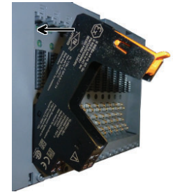
Fig-5: CHARM Terminal Block installation
