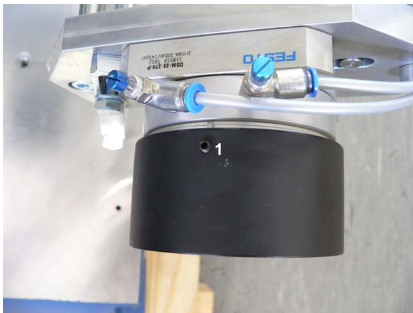
Fig. 2-6 Attach the cover cap to the foil forwarder (view from above)
