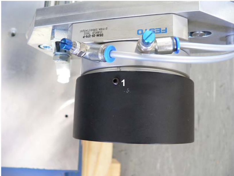
Fig. 4-5 Attaching the cover cap to the foil forwarder (view from above)
