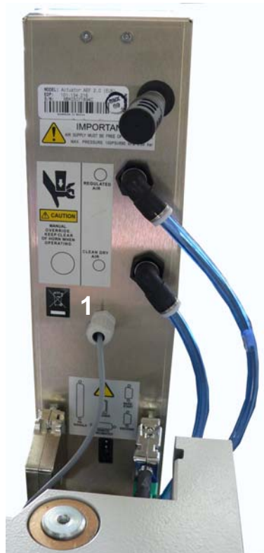
Fig. 4-1 Connection for solenoid valve located on back of actuator
