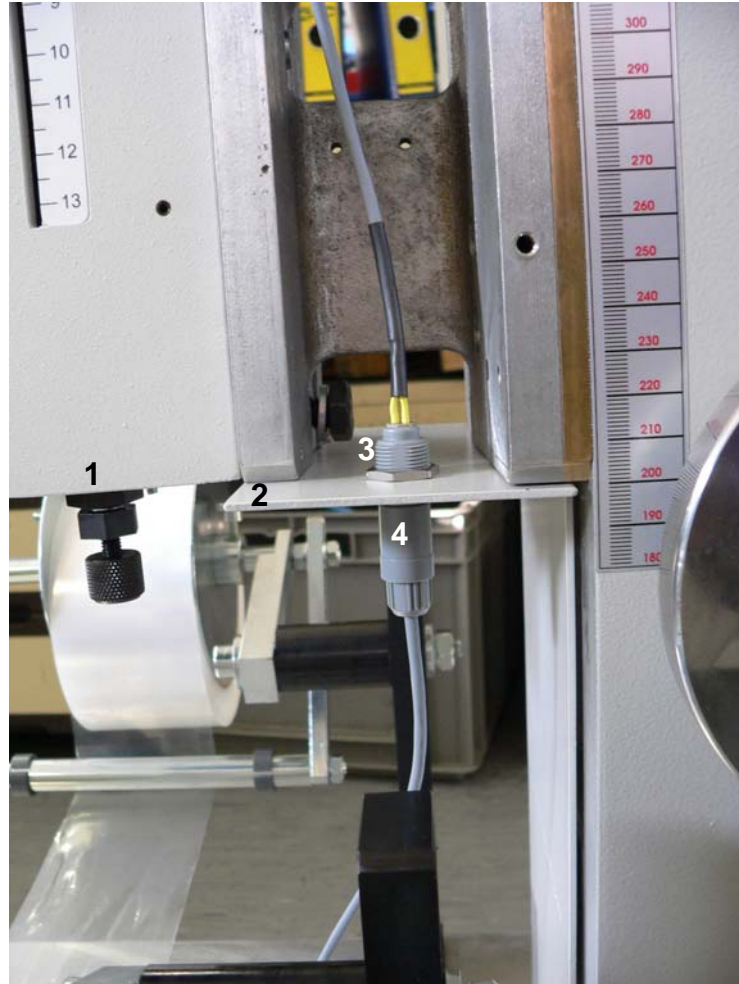
Fig. 4-2 Cable lead through - solenoid valve
