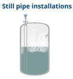
Measurement in still pipes commonly found in turbulent low dielectric fluids or where multiple internal obstacles are present.
