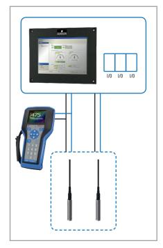
**Digital HART® communication protocol** enables remote control and diagnostics to reduce unnecessary work in high risk area.
