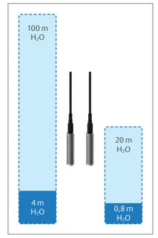
**25:1 Rangeability** allows one and the same transmitter for all tank level applications.
