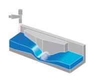
Use the Rosemount 1408A for volume flow measurement of water and wastewater in open channels.
