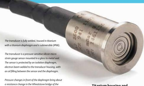
a resistance change in the Wheatstone bridge of the transducer. This change in the Wheatstone bridge is transmitted to the amplifier as a change in the signal.
