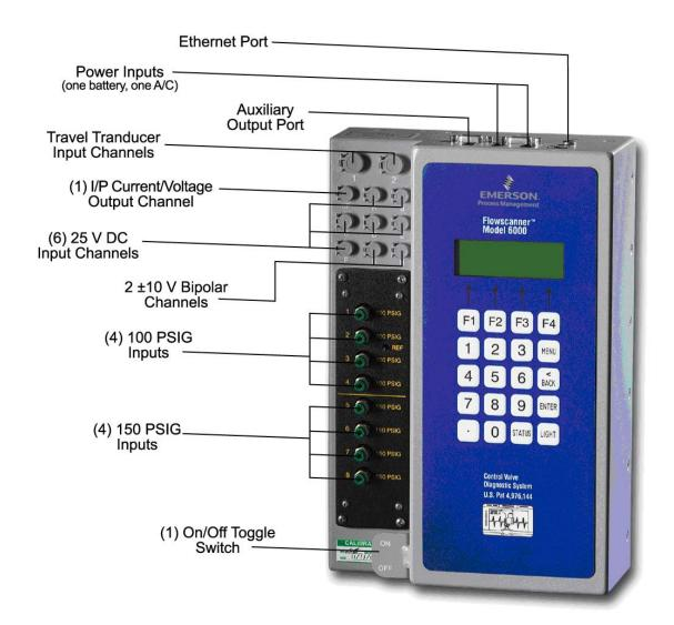
Figure 9. The FlowScanner 6000's input/output connections.
