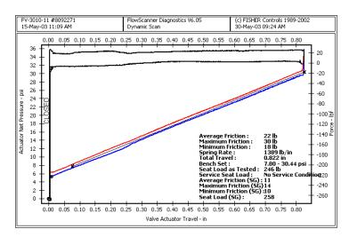
The FlowScanner software provides easy scaling of the strain gauge output to force units, and the resulting data can be plotted and analyzed on its own, or overlaid and compared to the simultaneously measured pressure-based analysis.
