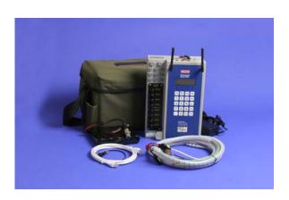
**Figure 1.** The FlowScanner 6000 housed in its convenient padded canvas operating bag (left), and analyzing a control valve in a field situation (right).
