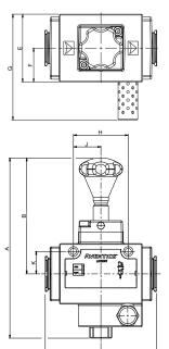
Note: When the knob is pushed down (Closed position), the lockout shaft extends out of the bottom by 12,2 mm. The lockout hole diameter in the shaft is 11,2 mm. These measurements are the same for the standard Lockout and the Slow-Start version.
