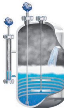
Figure 2.1.1 GWR can handle disturbing objects and tough process conditions. It can be installed directly in the tank or in a by-pass chamber
