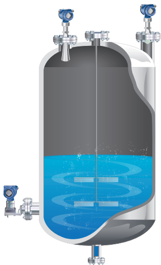
Figure 4.8.1: Level measurement in a tank with agitation
