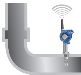
Figure 4.18.5: A wireless level detector detecting whether there is liquid or not in the pipe
