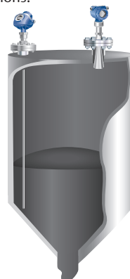
Figure 5.2.6: Fly ash level with non-contacting radar and guided wave radar
