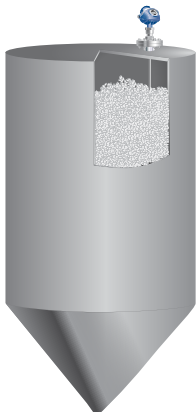
Figure 5.2.8: Polyethylene storage silo with guided wave radar
