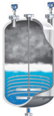
Figure 2.2.1 Non-contacting radars with different antennas to fit different applications.
