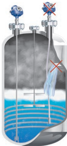
Figure 6.10.1: Mounting position in liquids
