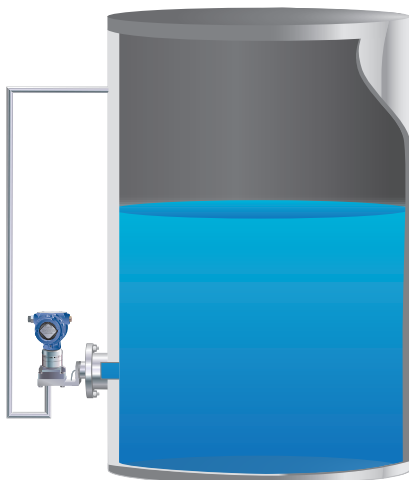
Figure 9.1.1: Illustration of a wet leg installation
