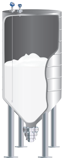
Figure 5.2.2: Flour silo with guided wave radar and non-contacting radar
