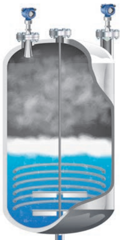
Figure 4.9.1: Reactor vessel level with non-contacting radar
