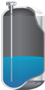
Figure 6.13.8: GWR measuring level in stilling well
