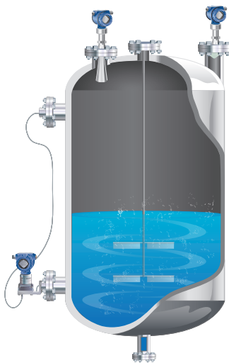
Figure 4.8.2: Slurry level with non-contacting radar and differential pressure
