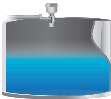
Figure 2.3.1 Illustration showing an ultrasonic transmitter
