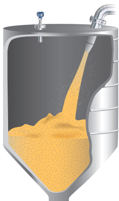
Figure 5.2.4: Non-contacting radar on grain silo
