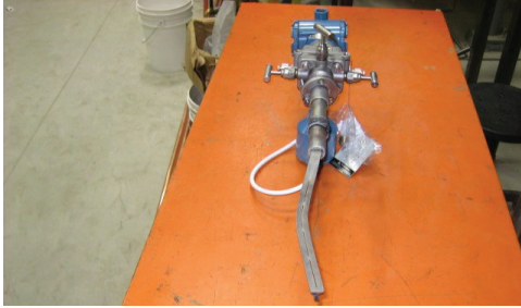
Figure 10.1: Rosemount 485 Annubar Primary Element damaged by improper installation.
