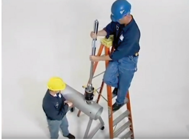
Figure 10.36: A simple hand-operated hot tapping machine.
