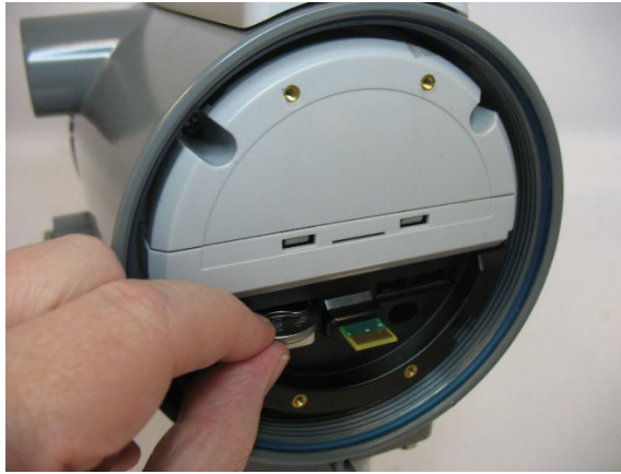
Figure 4-6. Removing/Replacing the Coin Cell Battery
