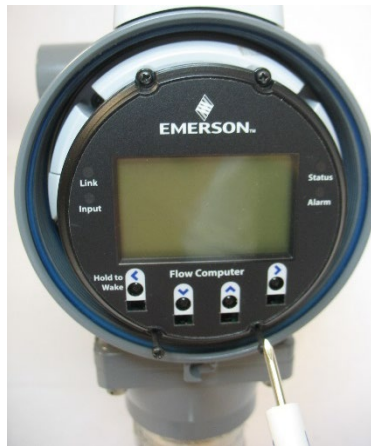
Figure 4-3. Captive Fastening Screws
