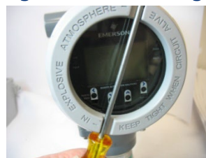
Figure 2-5. Removing or Tightening the End Cap with Long Screwdriver
