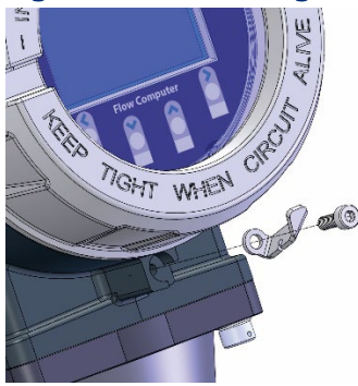
Figure 2-4. Retaining Clamp and Screw
