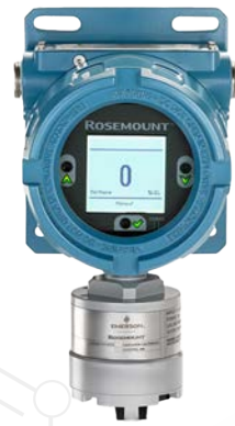
Figure 14: Fixed point combustible and toxic gas detectors use multiple sensor technologies, such as infrared, catalytic bead and electrochemical. The Rosemount 925FGD Fixed Gas Detector (left) can detect all flammable gases and common toxic gases. Rosemount 935/936 Open Path Combustible and Toxic Gas Detectors (right) use infrared and ultraviolet technology to detect hydrocarbon and toxic gases, including methane, propane, ethylene, hydrogen sulfide and ammonia.
