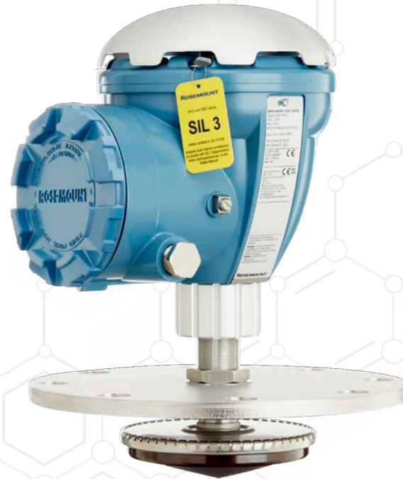
Figure 5: The Rosemount 5900 Radar Level Gauge can be proof-tested safely and remotely from the control room using Rosemount TankMaster™ Inventory Management Software that allows an operator to perform one or several proof-tests. Following a guided process, proof-testing can be done in less than five minutes, and afterwards an automatic report is generated which specifies the details of the test and confirms success result i.e. Pass/Fail.
