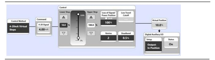
The Lower Virtual Stop can be configured from 0% to 99.9% but must be less than the Upper Virtual Stop. When the Lower Virtual Stop is greater than 0% the actuator will stop closing at the Lower Virtual Stop value. For instance, if the actuator is calibrated from 4-20mA and the Lower Virtual Stop is configured to 10%, a value of 5.6mA or less will drive the actuator to a position of 10% but the actuator will not close further.
