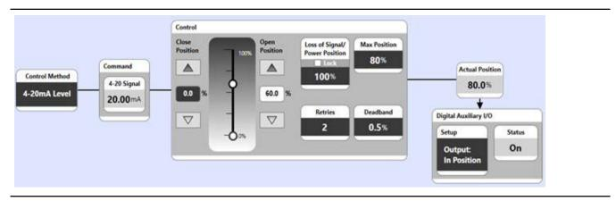
When the commanded position is greater than the Open Position, the actuator will open no further than the value of the Analog Level Max Position. For example, if the Open Position is configured to 60% and the Max Position is set to 80%, a command value from 13.6mA to 16.8mA will open the actuator to the equivalent position (60 to 80%). A commanded value of 16.8mA or greater will open to 80% but no further.
