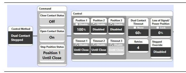
Each of the Positions can be configured to a value between 0 and 100% or Disabled, at least one Position must be enabled. Each Timeout can be configured to a value between 1 and 60,000 seconds or Disabled. At least one Timeout for an enabled Position must be Disabled (Until Close) and Timeout 3 is always Disabled.
