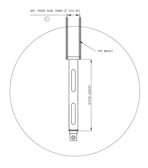
1 FOR CLEAN PRODUCTS ONLY. MIN PIPE SIZE FOR HIGH VISCOSITY PRODUCTS IS 3" SCH 40-80. THE ROSEMOUNT 765 IS NOT RECOMMENDED TO BE INSTALLED IN STILL PIPE FOR WAXY CRUDE OILS.
