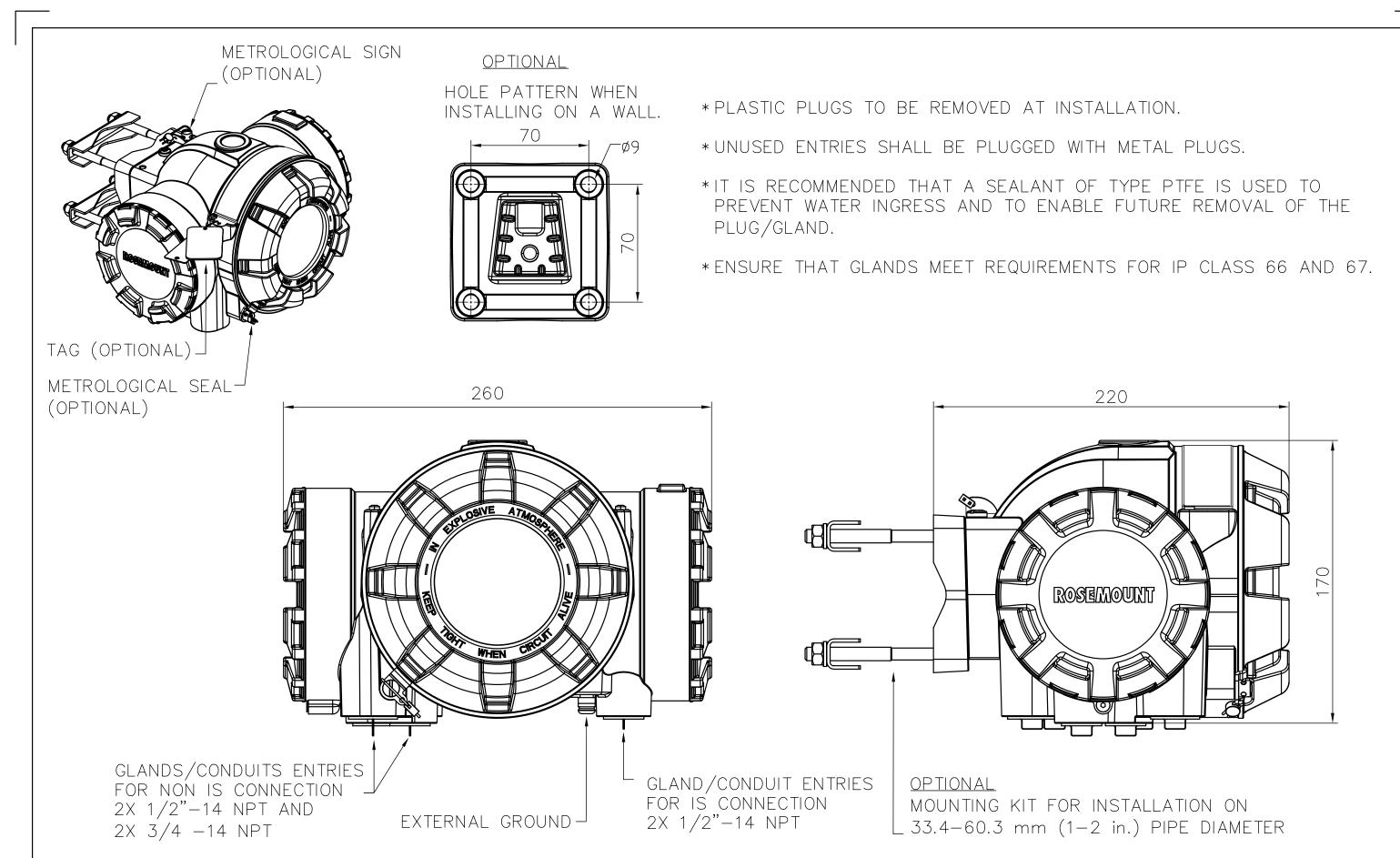
PLASTIC PLUGS TO BE REMOVED AT INSTALLATION.
