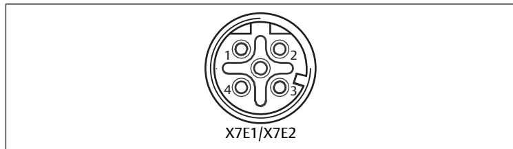
Fig. 3: Fieldbus connection pin assignments
