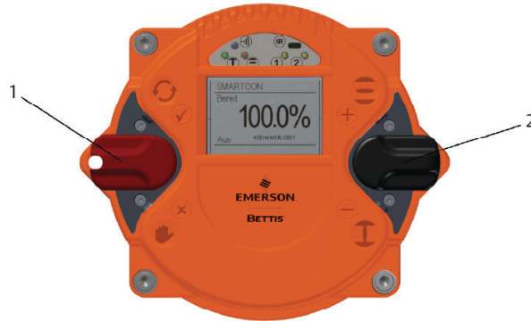
Figure 11 Switches in Center Position
