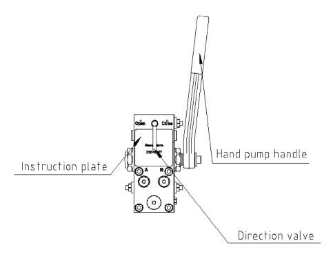
Description of the hand pump emergency operation can be found on the instruction plate mounted on the hand pump. The emergency description for the double line actuators is as follows:
