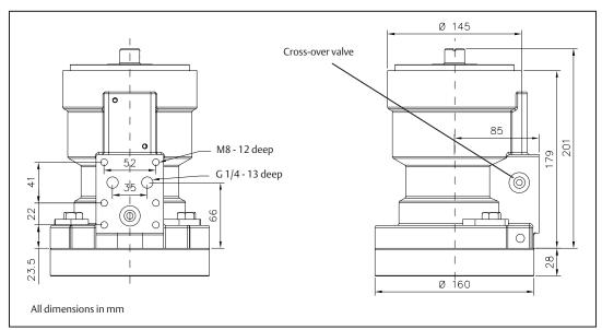
Actuator shown in closed position. A port: Close (clockwise seen from above), B port: Open.
