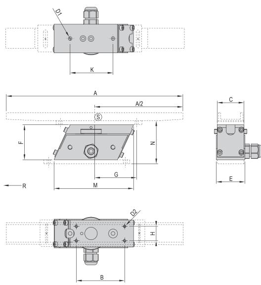
R = Feeding direction S = Track center of gravity
