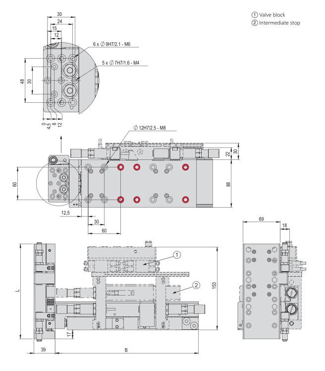
Bores can be screwed through. For additional and differently aligned bores that can be screwed through, see catalogue HT components linear
